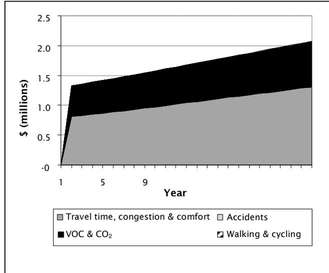
Figure A.14 Average time profiles of undiscounted costs for four bridge renewal projects
