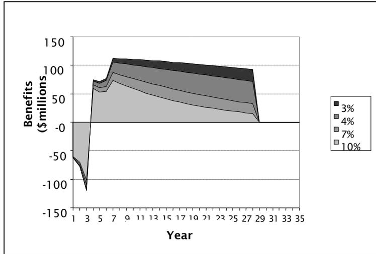
Figure 12.11 Discounted benefit and costs streams to year 80 for motorway construction projects
