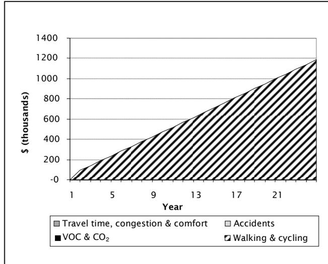
Figure A.19 Average time profiles of undiscounted costs for five new and improved walking network projects
