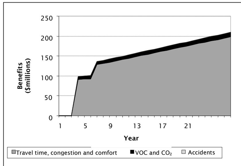
The benefit streams of motorway construction projects (figure 12.1) are characterised by a significant delay caused by construction and are measured in the hundreds of millions of dollars annually. They are predominantly comprised of travel time savings and congestion savings, and have strong linear growth projections.
