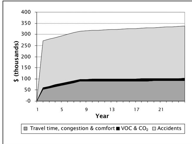
Figure A.12 Average time profiles of undiscounted costs for nine safety improvement projects
