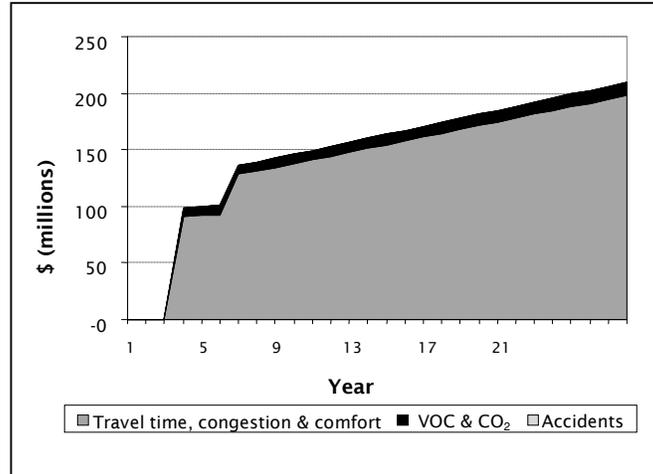
Figure A.2 Average time profiles of undiscounted costs for two motorway construction projects
