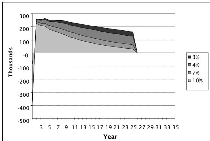
**Figure C.5** Discounted benefit and costs streams projected uniformly to year 80 for safety improvement projects
