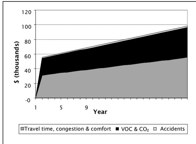
Figure A.4 Average time profiles of undiscounted costs for 50 seal extension projects
