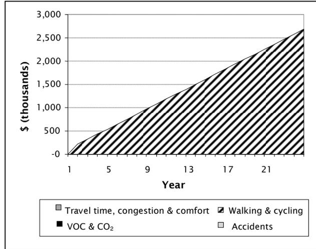
Figure A.10 Average time profiles of undiscounted costs for 10 new and improved cycling network projects
