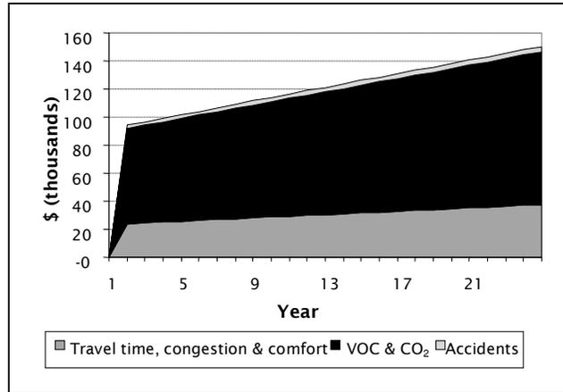
Figure A.6 Average time profiles of undiscounted benefits for 37 pavement smoothing projects
